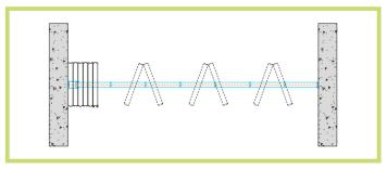
When remote storage is not required, the center-hung panels hinged in groups of two or three, are the ideal solution for quicker and easier set up, than omni-direction panels. Optional hinging is available to accommodate moldings or other decorations. Acoustical ratings are the same as omni-direction panels.
